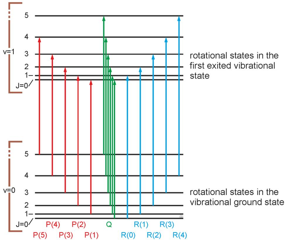
Abbildung 3: rotational-vibrational transitions
