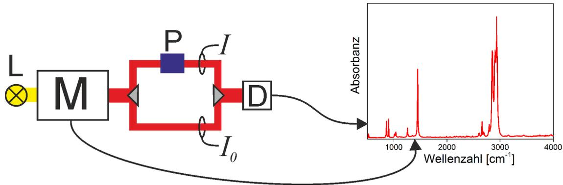
Abbildung 1: Sketch of a classical infrared spectrometer. The monochromator (M) selects the wavelength  $\lambda$  from the broad band light source (L) by rotating a diffraction grating in the monochromator housing. The light is then split into paths: sample beam (intensity  $I$ ) and reference beam (intensity  $I_0$ ).  $I$  and  $I_0$  are measured by the detector (D). The quotient  $I/I_0$  constitutes the y-axis of the spectrum, the position of the grating is the x-axis
